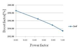
**Fig: 10.** Experimental Result of Relationship between Voltage Boost Ratio and Load Power Factor
