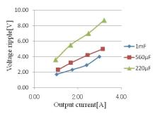
**Fig: 7.** Experimental Result of Relationship between Ripple Voltage of DC Capacitor and Output Current for Different Values of Capacitance.
