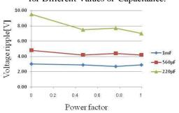
**Fig: 8.** Experimental Result of Relationship between Ripple Voltage of DC Capacitor and Load Power Factor for Different Values of Capacitance.
