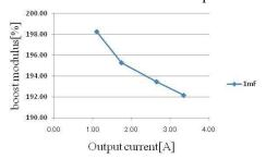
Fig: 9. Experimental Result of Relationship between Voltage Boost Ratio and Output Current.
