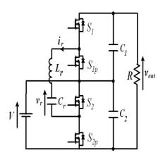
Fig: 2(a). Circuit Configuration.
