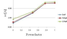
Fig: 6. Experimental Result of Relationship between Resonant Current and Load Power Factor for Different Values of DC Link Capacitor
